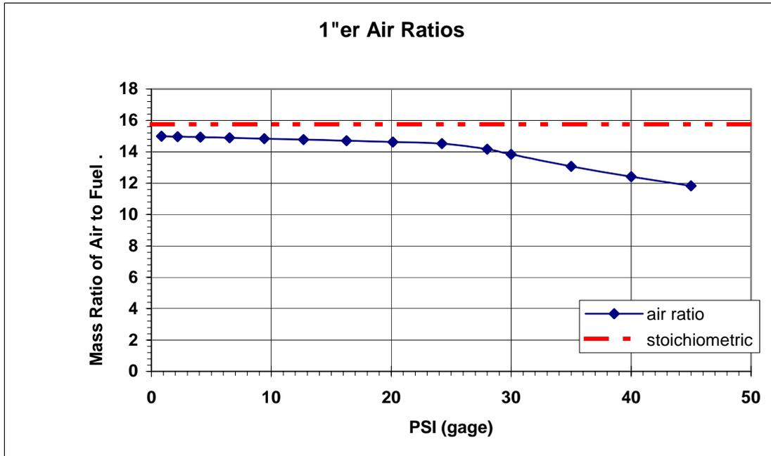
At pressures above about 27 PSI for this burner, the amount of air drawn in doesn't increase quite as fast as the fuel increases. (Larger burners will generally reach the sonic flow condition at lower supply pressure levels.) Thus operating in the sonic range is not recommended unless efficiency is not an issue in your application.
